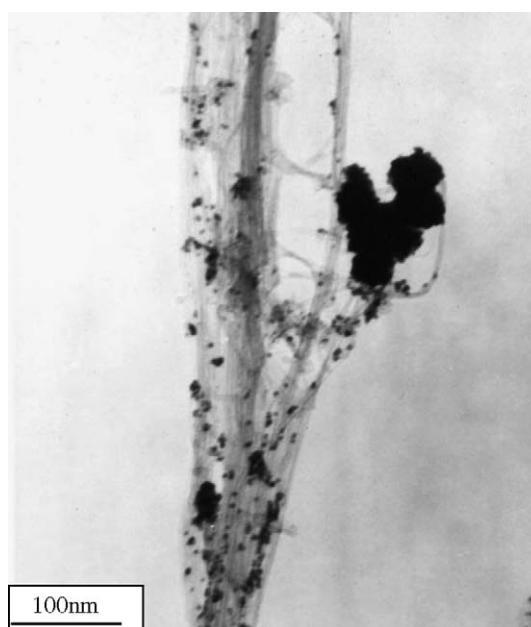
Fig. 4. Transmission electron micrograph (TEM) image of Pt/SWNT composites.
